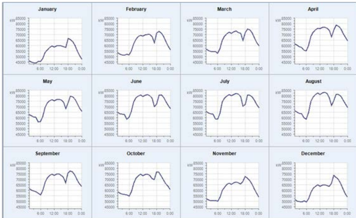
Figure 4-16: Representative System Load Curves by Month
